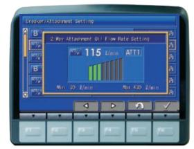
Fully integrated tool control. Up to 15 tool presets for oil flow and pressure.
